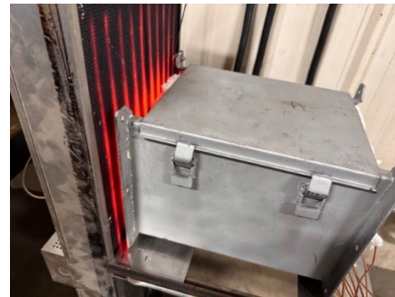
Figure 6. Experimental infrared heating setup.
