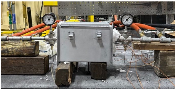
Figure 4. Experimental fluid setup for hot oil, hot water, and jet water.
