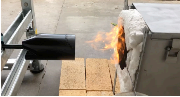
Figure 3. Experimental direct flame setup.
